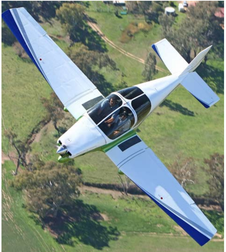
NOT SO SQUEEZY The Brumby's wide cockpit, divided by a centre console, affords both pilots reasonable personal space.
