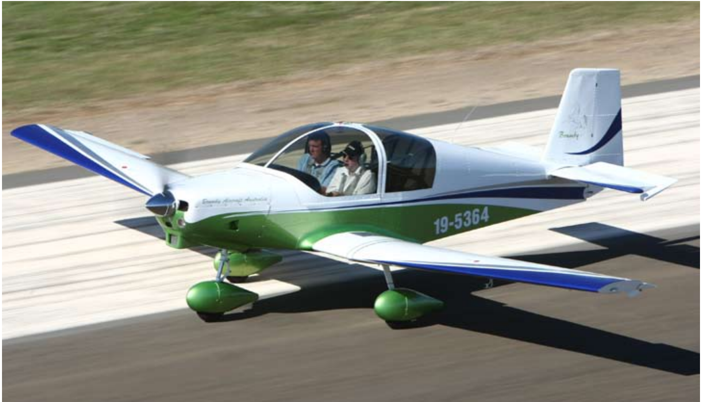
HORSEPOWER The test flight Brumby is powered by a Jabiru 3300 with options of Jabiru 2200, Rotax 912 and Continental O-200D powerplants available.
